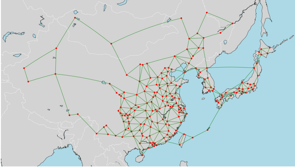
(b) East Asian network on the 200 settlements as nodes (larger cities chosen with bigger probability), with \sim 500 links, containing the MST
